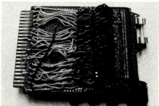
FIG. 3—UNDERSIDE VIEW REVEALS WIRING. The VIC-20 expander makes a good one-weekend project that will reward you with years of added convenience.
